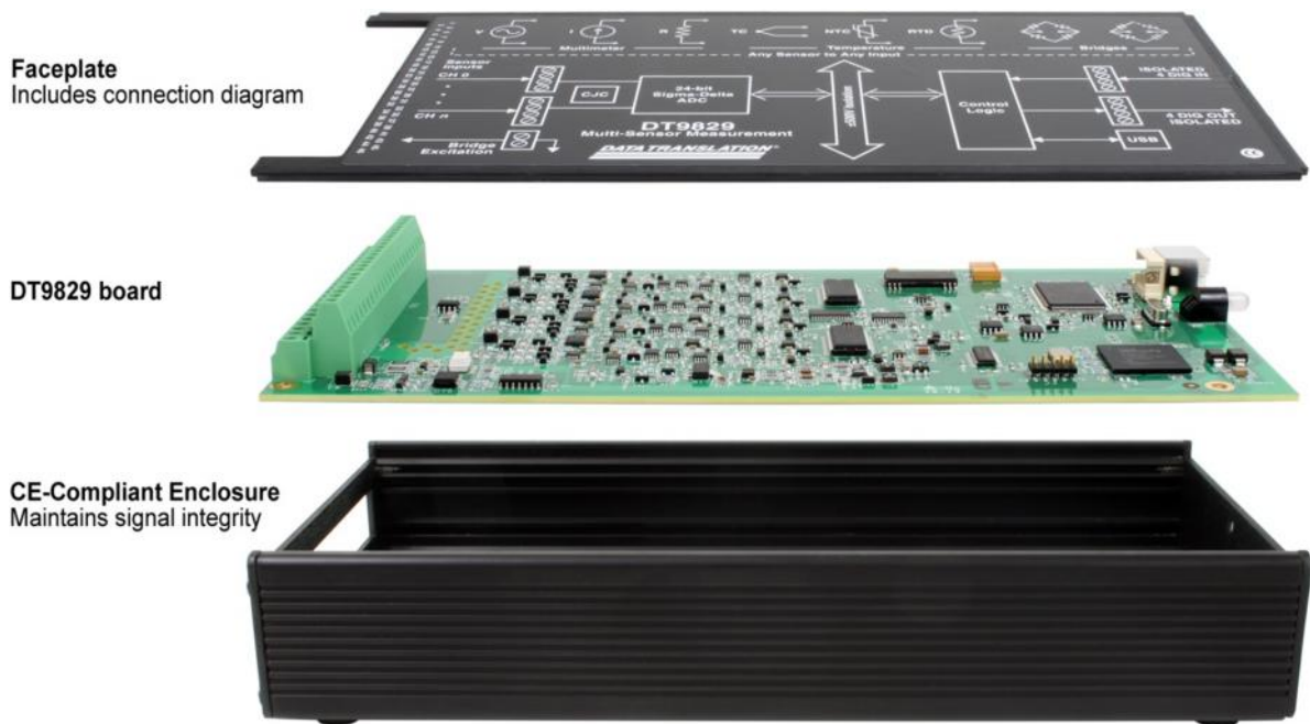
Figure 4. Exploded View. The DT9829 case packages the DT9829 in a CE-compliant enclosure.
